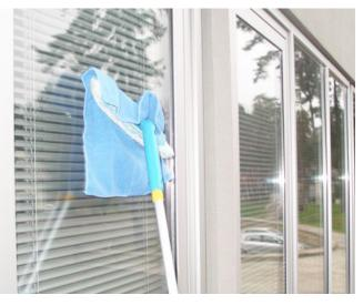
plane (polish) structure for polishing coated surface. Both cloths must be prepared from 20% polyamide and 80% polyester and density not less 250g/m2
